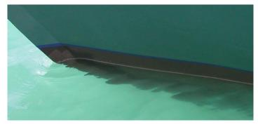
1 Hull partially or completely covered in slime fouling. Absence of any macrofouling.
