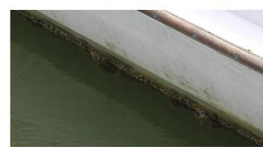
Very heavy fouling. 41 – 100 % of visible hull surface covered by macrofouling or filamentous algae. Usually remaining area covered in slime.
