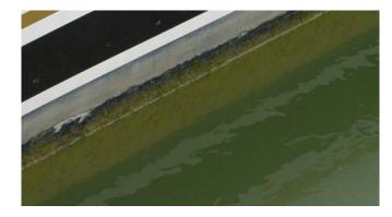
2 Light fouling. 1 – 5 % of visible hull surface covered by macrofouling or filamentous algae. Usually remaining area covered in slime.
