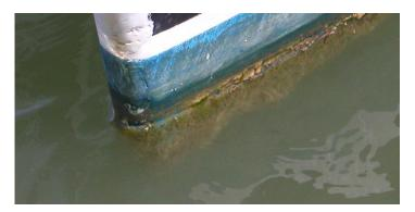
Considerable fouling. Macrofouling clearly visible but still patchy. 6 – 15 % of visible hull surface covered by macrofouling or filamentous algae. Usually remaining area covered in slime.
