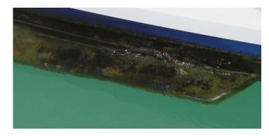
4 Extensive fouling. 16 – 40 % of visible hull surface covered by macrofouling or filamentous algae. Usually remaining area covered in slime.
