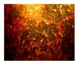
Very heavy fouling. 41 – 100 % of visible hull surface covered by macrofouling or filamentous algae. Remaining area often covered in slime.
