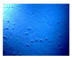
1 Hull partially or completely covered in slime fouling (biofilm). Absence of any macrofouling.
