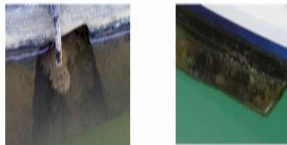
Considerable fouling. Macrofouling clearly visible but still patchy. 6 – 15% of visible hull surface covered by macrofouling or filamentous algae. Usually remaining area covered in slime.
